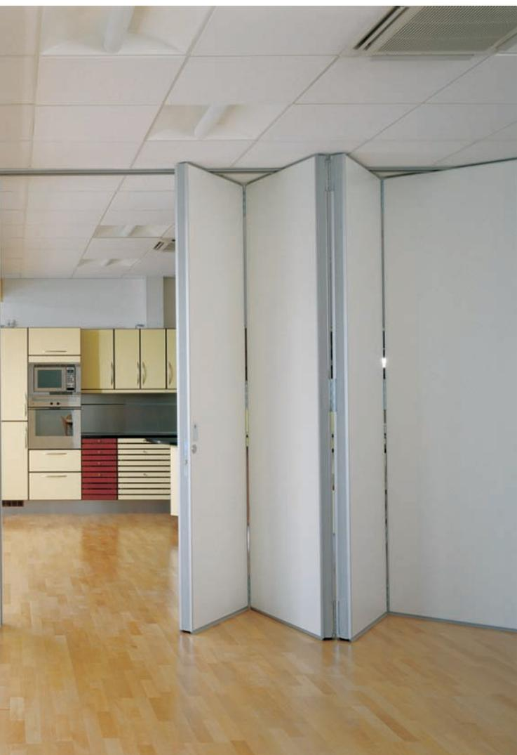
The top and the bottom of the panels are fitted with a rubber strip that seals tightly when the partitions are locked. The edges of the panels have a protective trim to prevent damage. As standard, the edge trims are produced in natural anodised aluminium, but they can also be supplied in other colours if required.
